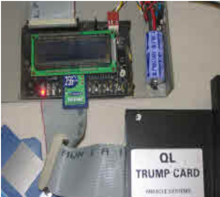
An uncased HxC SD card interface attached to a Trump Card QL.
